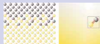
Compound material with covalent bonded titanium layer of \sim 30 nm thickness only; patented nanotechnology.
