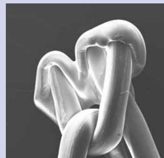
Laser-cut mesh edges result in rounded fiber ends, thus preventing micro traumata.
