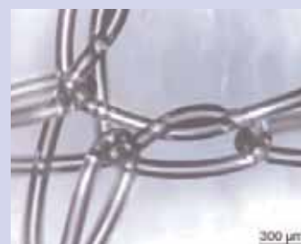
Smooth and flexible fiber with only 16 \text{ g/m}^2 provides optimized biocompatibility and patient comfort.
